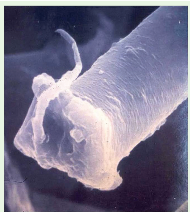
Figure 18-4. Scanning photomicrograph of nylon flock fiber with fibril on cut end that can be dislodged to form a respirable dust associated with flock worker’s lung. Data source: Burkhart J, Piacitelli C, Schwegler-Berry D, Jones W. Environmental study of nylon flocking process. J Toxicol Environ Health . 1999;57:1–23.
